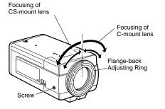
**Caution:** Tightening the screw by force will cause damage to the screw or deviation of focus.
